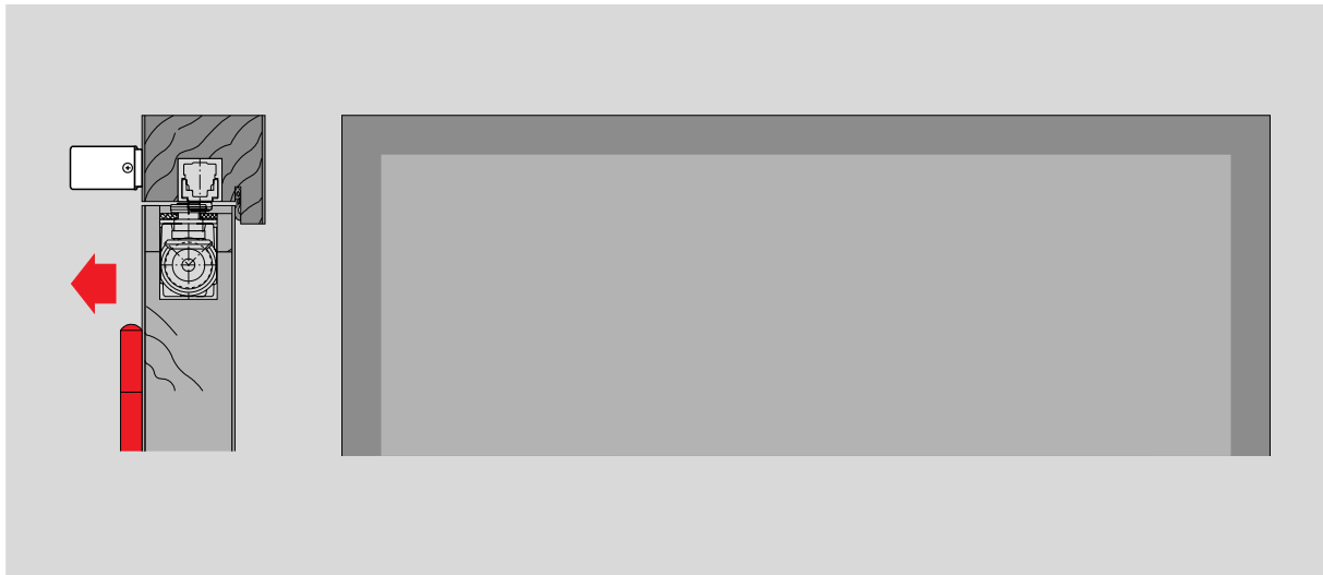
RMZ-K/S frame-mounted smoke detector on the pull side connected to an ITS 96 EMF Example: Anticlockwise-closing (ISO 6) door; mirror image applies to clockwise-closing (ISO 5) doors.
